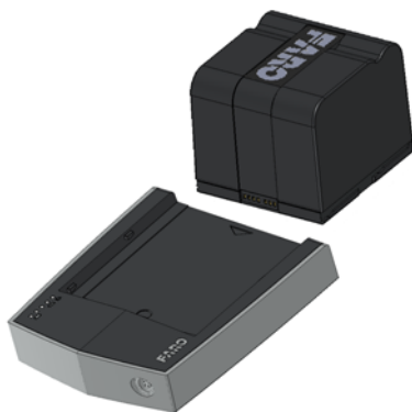
Figure 5-2 Placing the Battery on the PowerDock
