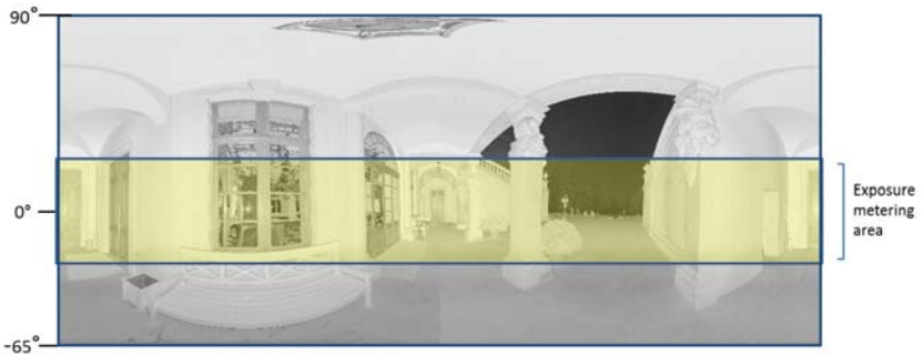
Figure 5-24 Full vertical scan area
