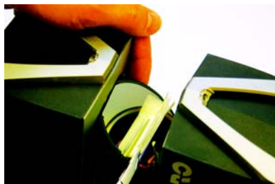
Figure 3-4 Cleaning the Mirror
