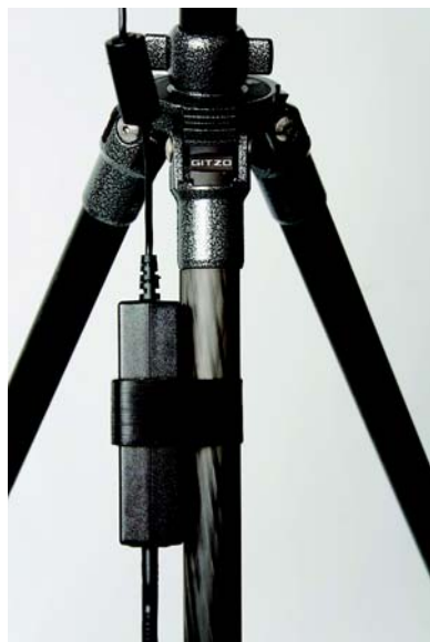
Figure 5-6 Power Supply Attached to the Tripod's Leg
