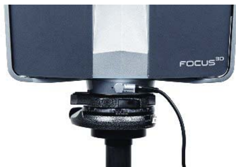
Figure 5-7 Power Supply Connected to Focus 3D X 130
