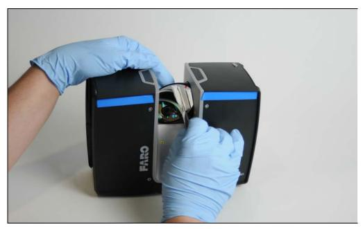
Figure 9-9: Cleaning mirror module with pad and isopropyl alcohol or cleaning fluid
