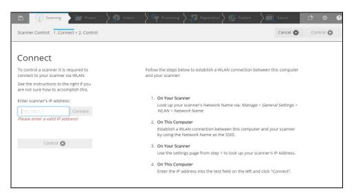
Figure 8-2: Connect page: Enter the IP address
