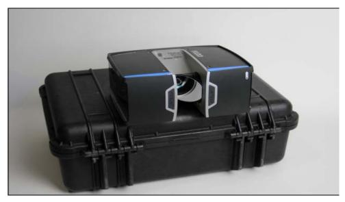
Figure 9-12: Transport box with laser scanner turned and laid on top, with the mirror module facing outwards
