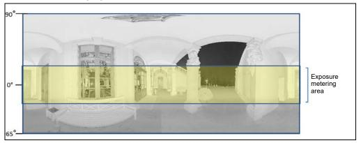
Figure 7-14: Exposure metering area (highlighted yellow) for the full vertical scan area
