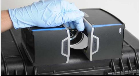
Figure 9-13: Fix the mirror with your finger tips to keep it in this position
