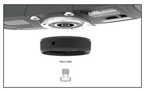
2. Put the S3 hex key (shown here in silver) as an interlock into one of the three openings of the threaded collar. Slightly turn the collar and find a spot where the hex key fits into one of the six openings of the inner ring. Make sure that the hex key actually went into one of the six openings of the inner ring.
