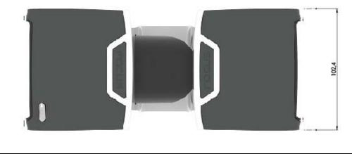
Figure 10-1: Scanner Dimensions
