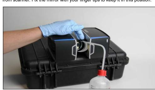
4. Turn the mirror module into vertical position, i.e., the mirror points away from scanner. Fix the mirror with your finger tips to keep it in this position.
