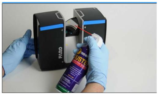
Figure 9-11: Dry pre-cleaning by compressed air or duster cleaning spray
