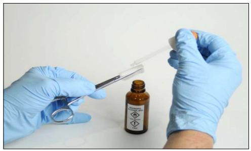
Figure 9-8: Soaking the cleaning pad
