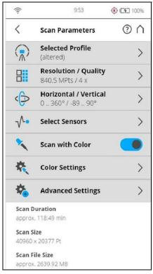
Figure 6-15: Change the Scan Parameters
