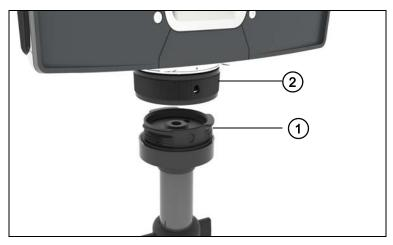
The Quick Release consists of two main parts: the base plate (1) to be put on top of the tripod's platform, and the mount plate (2) to be attached underneath the scanner. The Quick Release is packaged with two hex keys which are needed for mounting:
