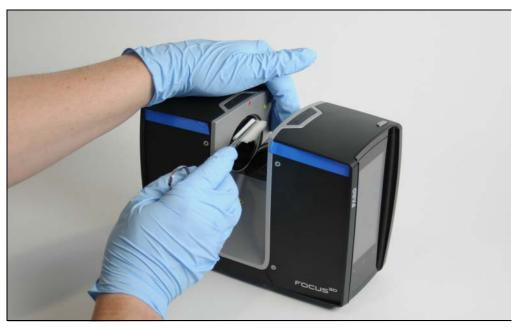
*Figure 9-10: Cleaning sensor cover with pad and* isopropyl alcohol o*r cleaning fluid*
