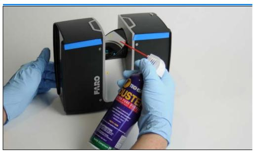
Figure 9-1: Dry pre-cleaning with compressed air or duster cleaning spray
