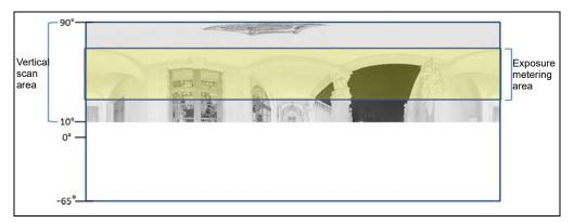
Figure 7-15: Exposure metering area for a limited vertical scan area set to e.g.,  $10^{\circ}$  to  $90^{\circ}$
