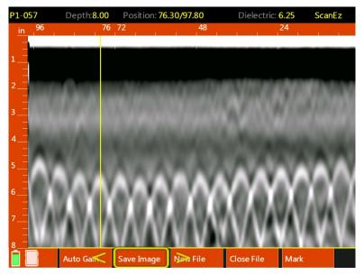
**4** Take a minimum of two survey lines in each direction and connect your marks to draw what is in the slab on the slab.
