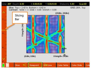
**Contrast:** Allows you to change the distribution of the color table along the amplitude scale. This is useful for highlighting certain areas of the data such as bright reflection from metals. The current color values are displayed above the grid image.
