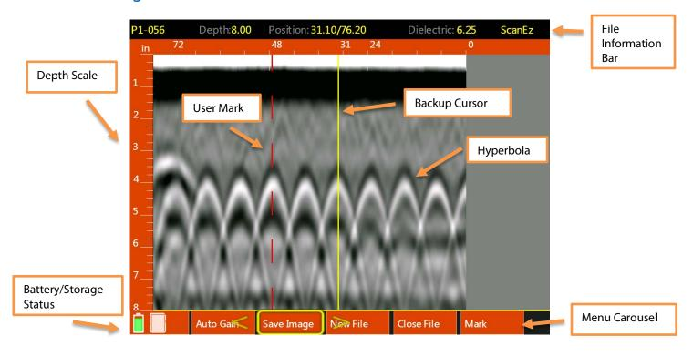
**5** If you haven't done so already, pull trigger to begin collecting data and roll the Mini XT across the concrete. The data image will be displayed in real time.
